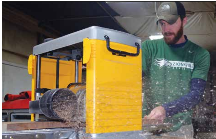
Above: Destined for future cabinetry projects, a wood plank is fed by Myers through the shop's planer. Staley and Myers refinish and build custom cabinets for homeowners in the Hendricks County area.
