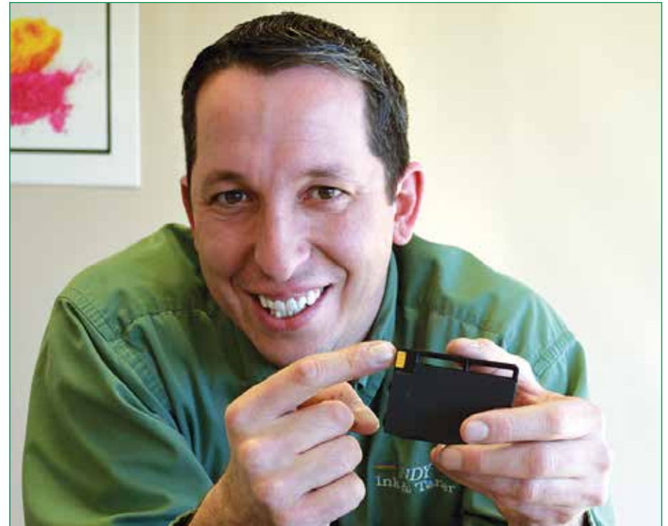
Indy Ink and Toner owner, Greg Platts, points out the tiny microchip installed on most new printer ink cartridges. Photos by Chris Cornwall
