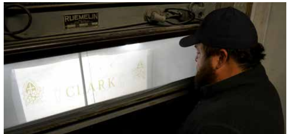
Bryce Hunt etches a stenciled pattern into granite with a high-velocity sandblaster. Photo by Chris Cornwall.
